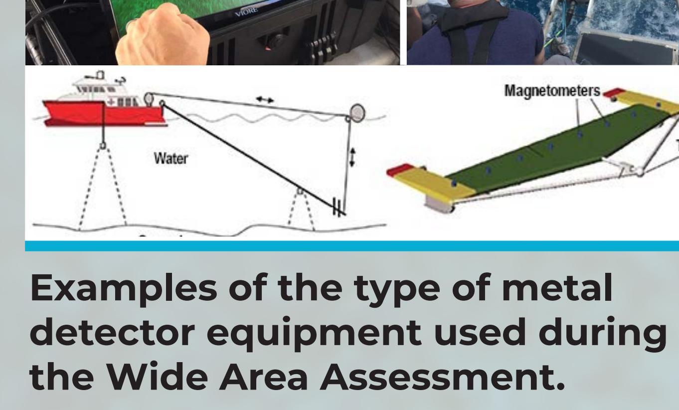
Examples of the type of metal detector equipment used during the Wide Area Assessment.
