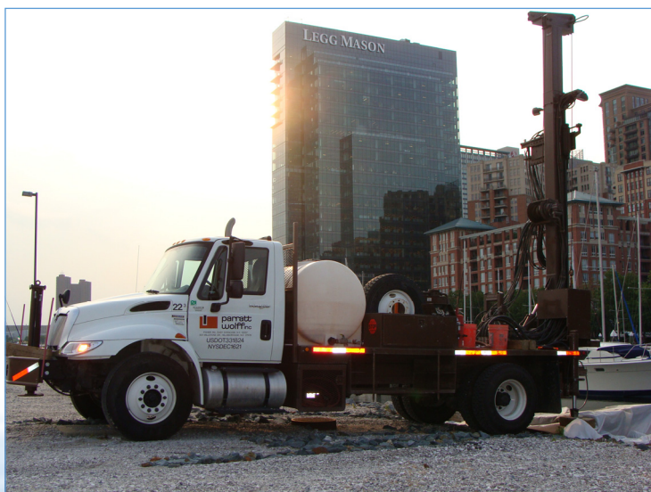
Drilling Rig Used for Monitoring Well Installation
