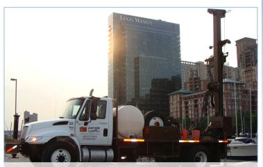
Photo of a drilling rig Used for monitoring well installation. Please do not approach the rig during operations.
