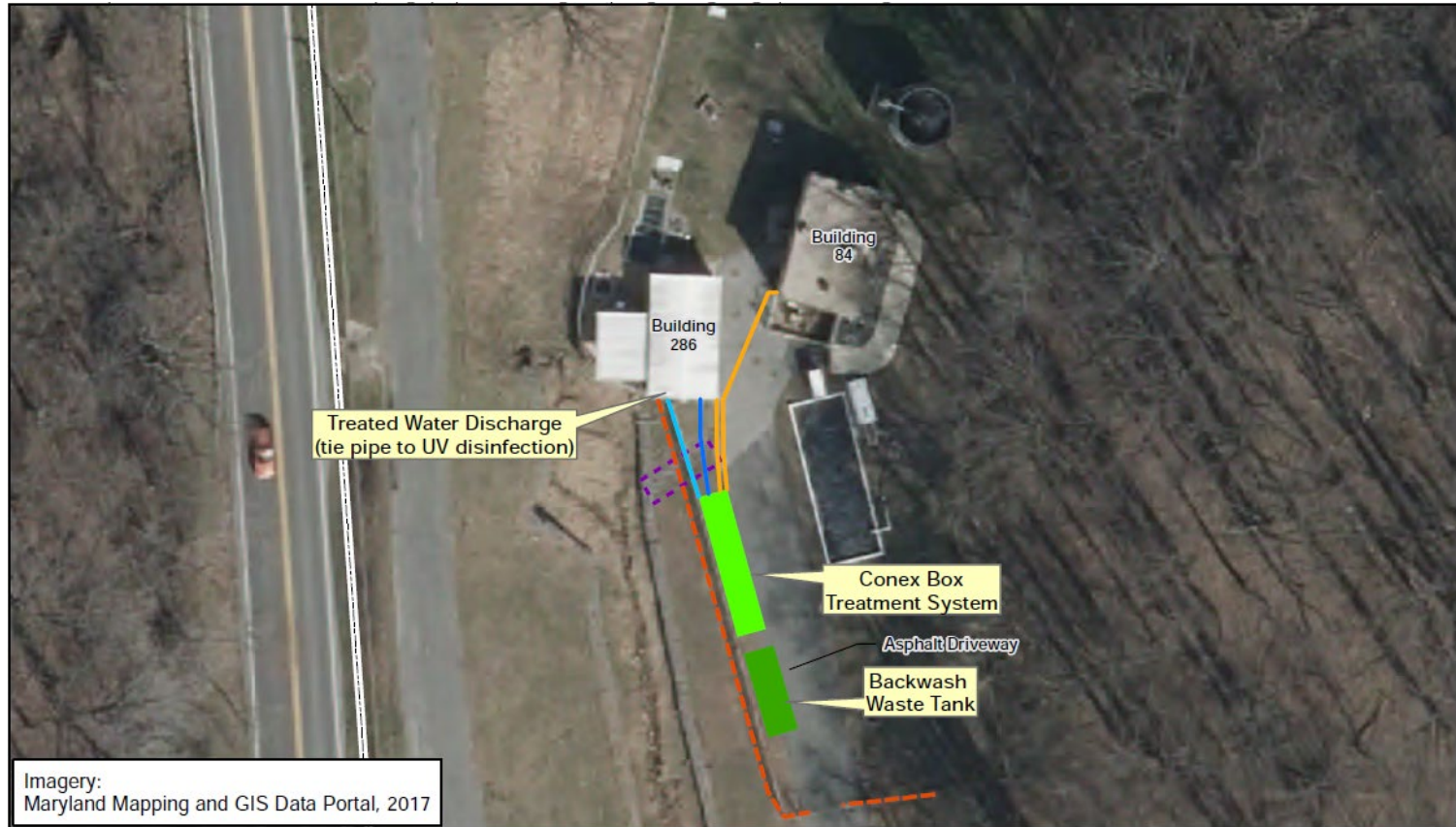
Figure 4-2 WWTP Treatment System Proposed Site Layout Basis of Design Memorandum for Interim Measures for PFAS Removal NRL-CBD Chesapeake Beach, Maryland
