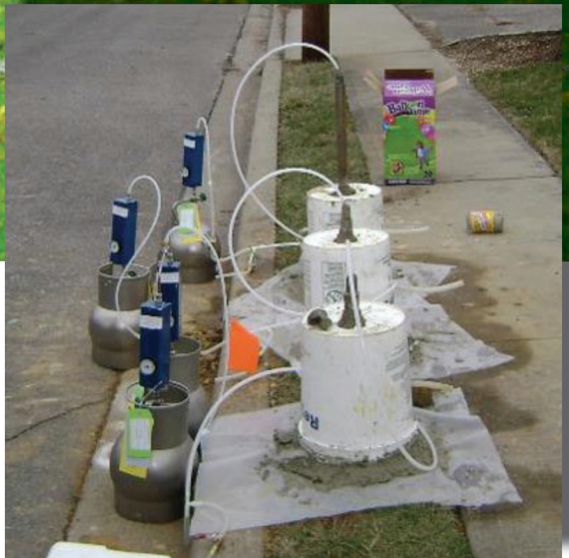
(Above) Technicians perform Soil Gas Sampling in a Nassau County residential neighborhood. Soil gas can be tested in different ways. The most common method uses a hollow metal rod that is inserted into the soil. To measure the soil gas holes are drilled and the rod is pushed into the soil. A pump draws the soil gas through the hollow rod into a sampling container or canister. The gas is then either analyzed by the testing equipment on-site or the sampling container is brought to an off-site laboratory for analysis.
