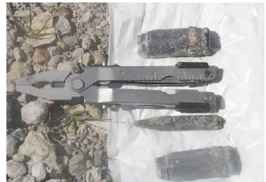
DU penetrator shown next to pliers
