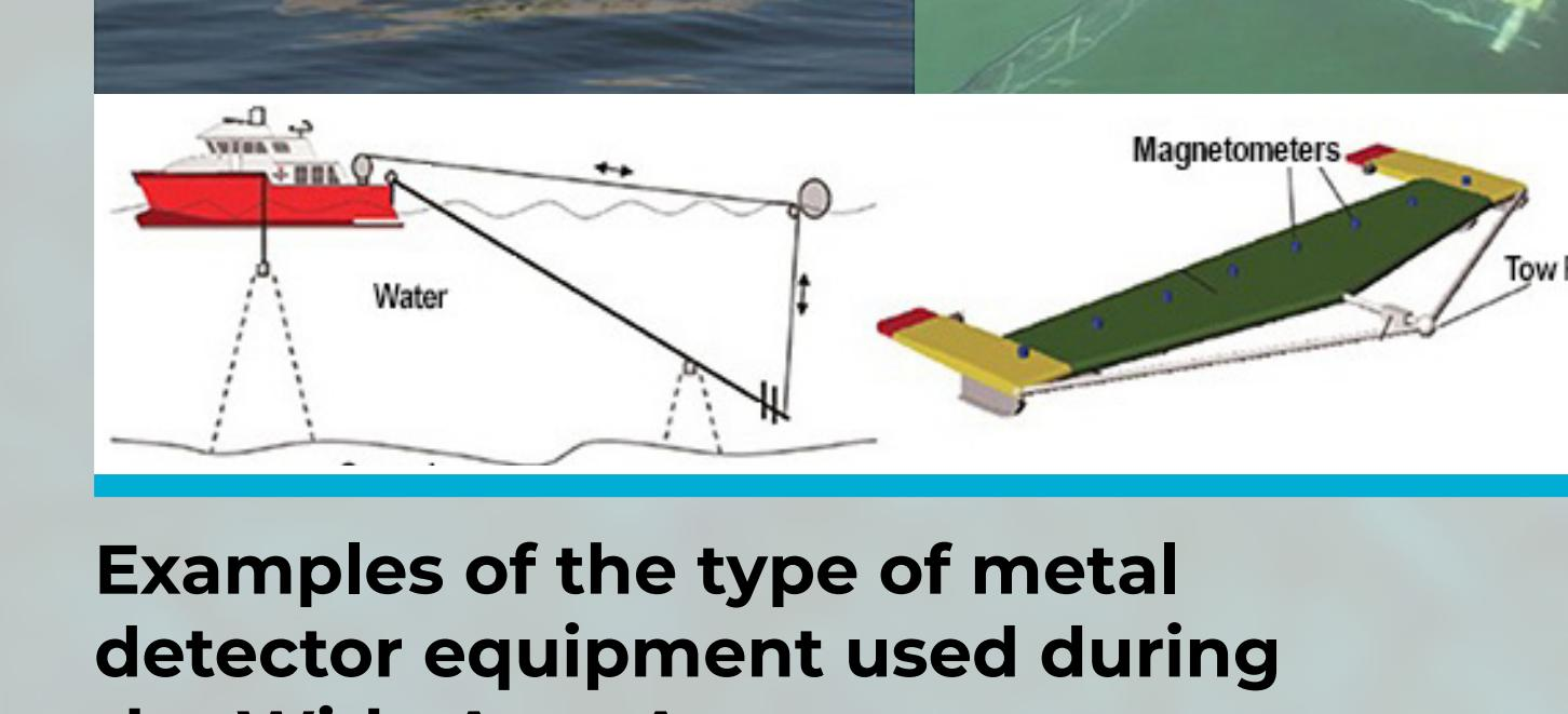
Examples of the type of metal detector equipment used during the Wide Area Assessment.
