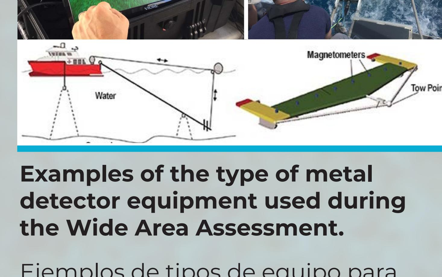
Examples of the type of metal detector equipment used during the Wide Area Assessment.
