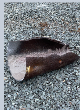
Water jet cutting an explosive-free munition
