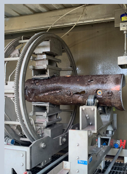
Water jet cutting an explosive-free munition
