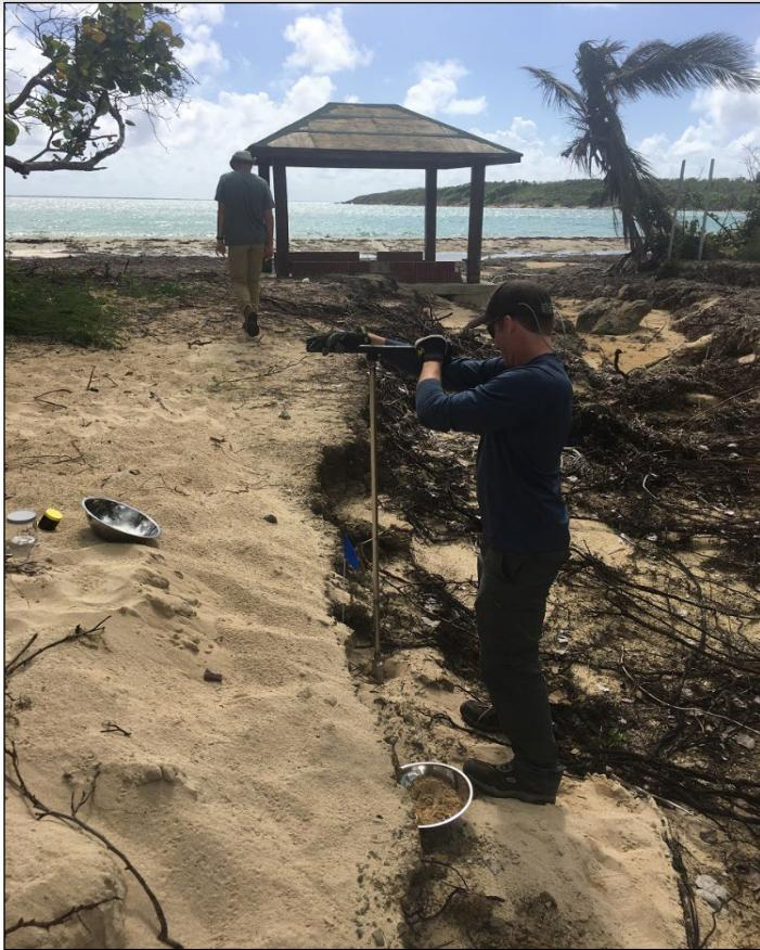
**Hand Augering to Collect Soil Samples**
