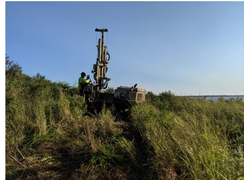
Groundwater sample collection with DPT rig
