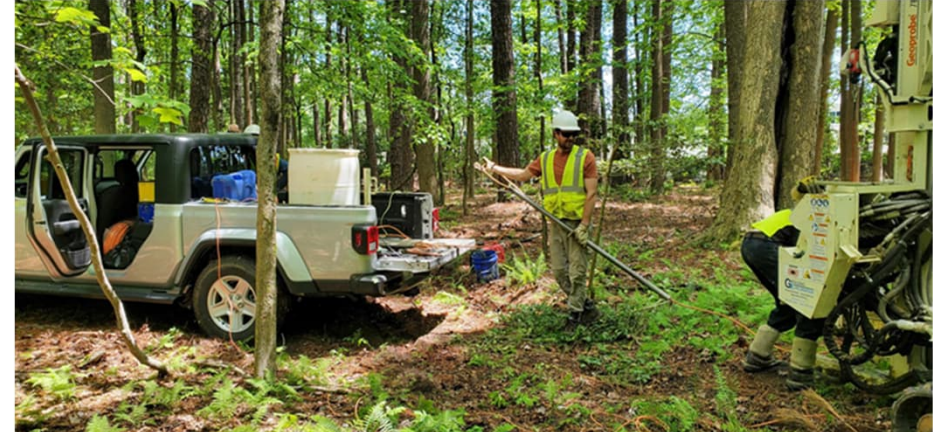
Hydrogeological data collection with HPT tooling
