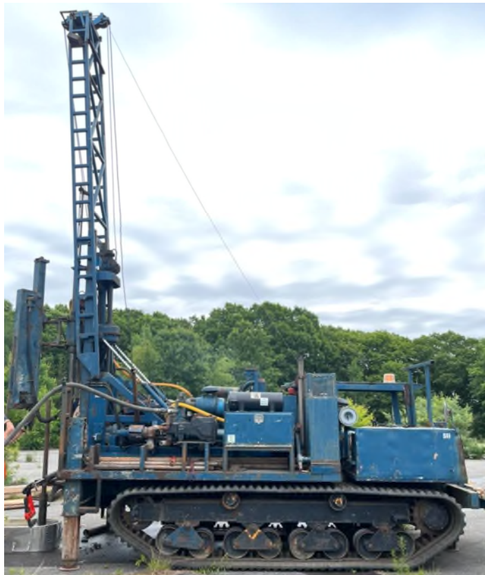
Photo 1: Type of drill rig that will be used to install shallow monitoring wells.
