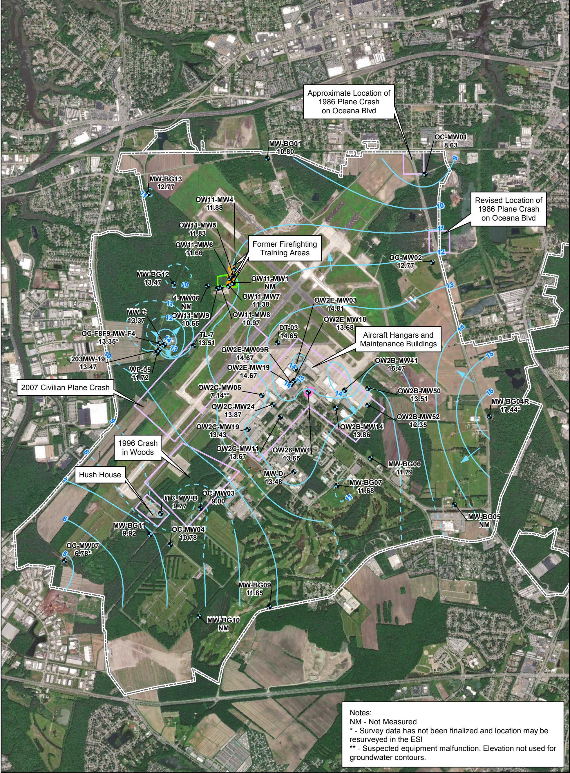
Figure 2 Columbia Aquifer Groundwater Elevation Contours - September 2018 NAS Oceana Virginia Beach, Virginia
