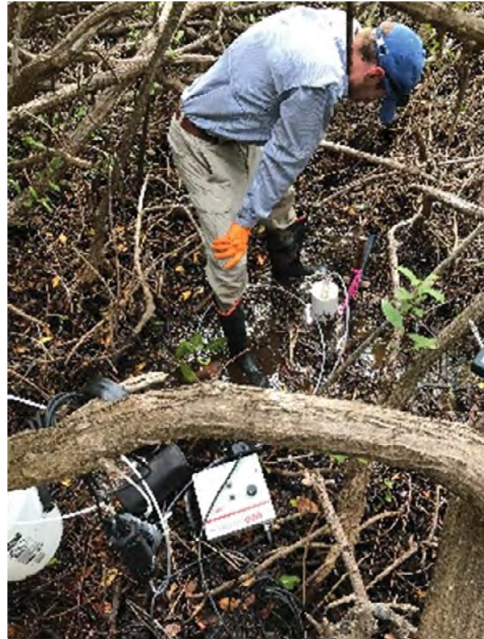
Surface water, pore water and sediment sampling
