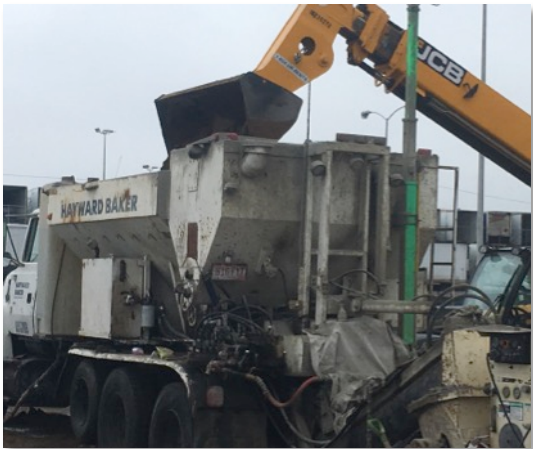
Batch-mix amendment ingredients in Elkin Mixer
