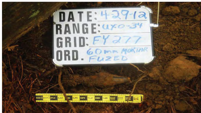
Live, fuzed High Explosive 60 mm mortar found on surface
