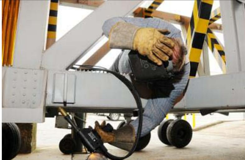
Figure 42: Before: Welder is in awkward posture to reach beneath work piece
