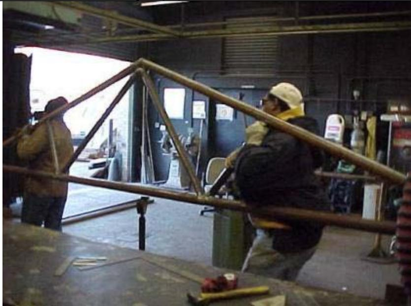
Figure 25 Manual lifting and carrying of fabricated work piece (US Naval Observatory)
