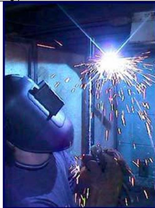
Figure 6 Welding above shoulder height
