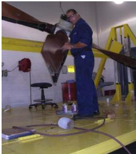
Figure 40: Fixture is height and angle adjustable
