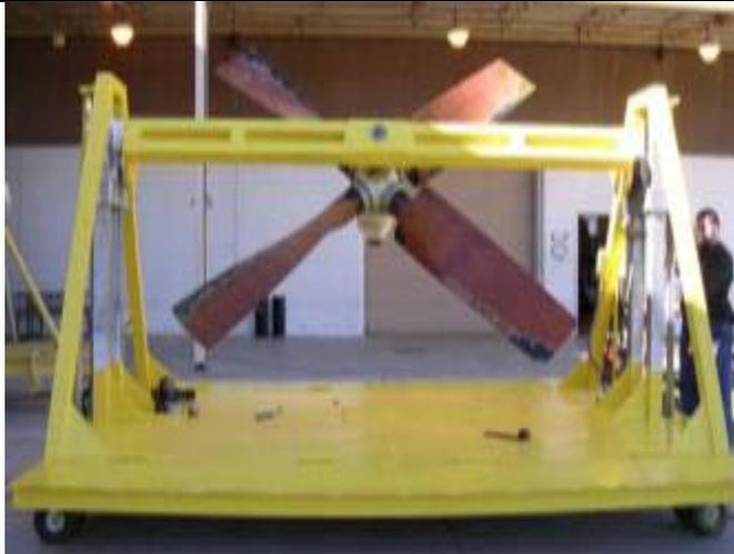
Figure 41: Propeller fixture
