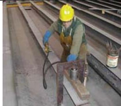
Figure 48: Welder using manual clamp method
