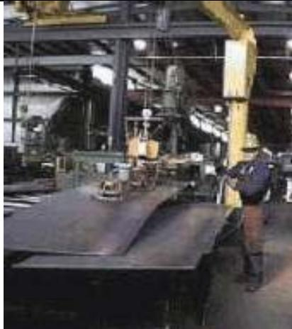
Figure 22: Suction manipulator used to move sheet metal
