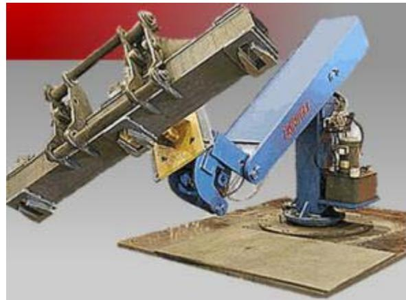
Figure 33 Rotating manipulator allows pieces to be held and manipulation in every direction.
