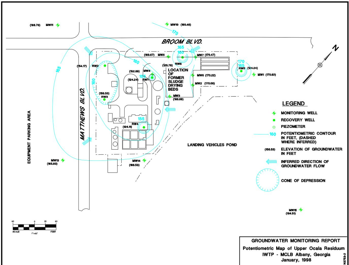
Figure 1. Monitoring Well Network for the Sludge Drying Beds
