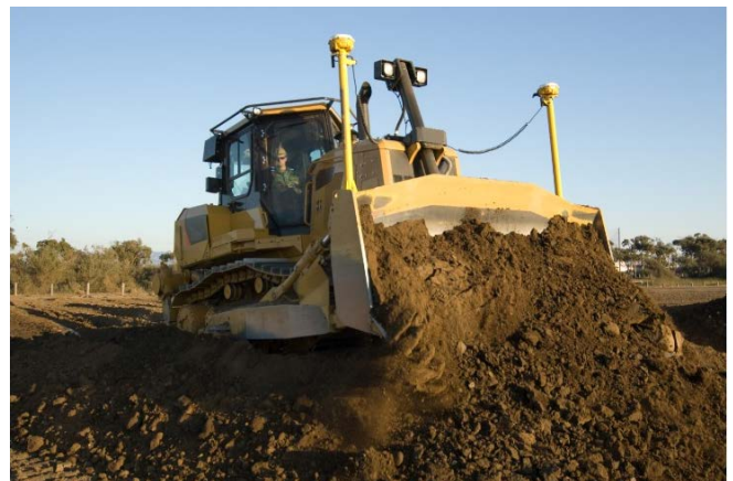
Diesel Electric Hybrid Dozer with Automated Blade Control
