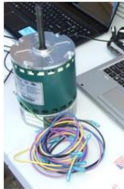
New ECM Green Motor Installed in Blower Prior to Demonstration
